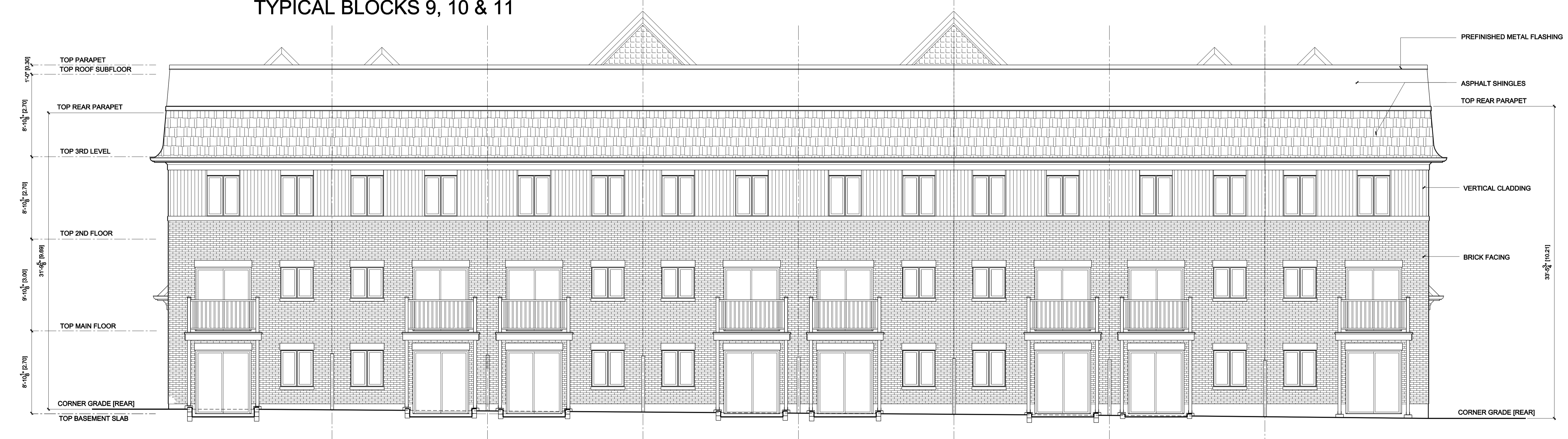
3 STOREY BLOCK REAR ELEVATION TYPICAL BLOCKS 9, 10 & 11
