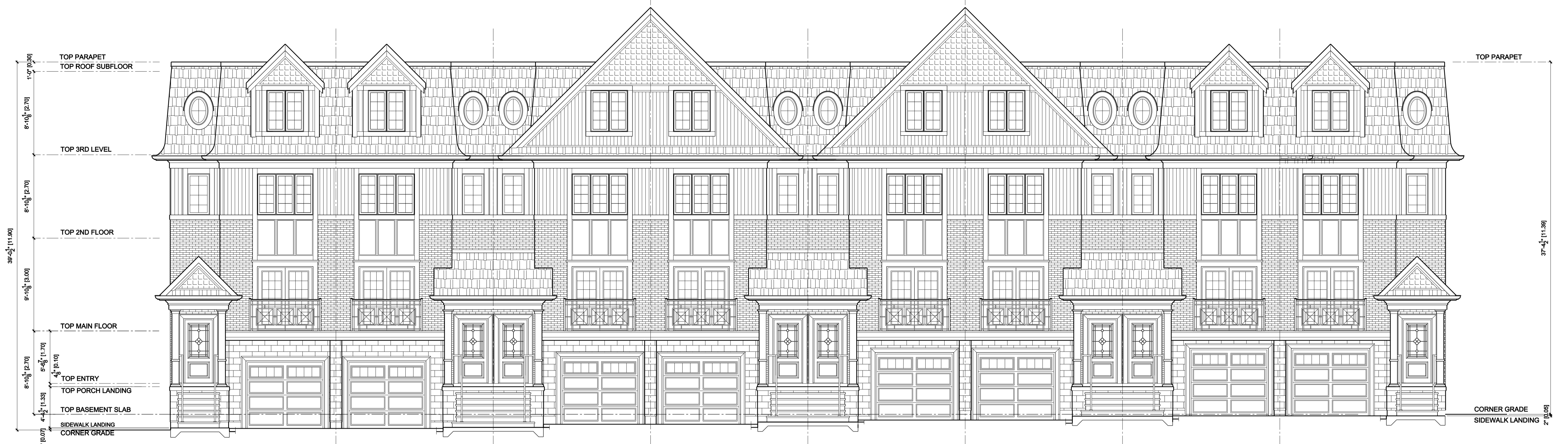
3 STOREY BLOCK FRONT ELEVATION TYPICAL BLOCKS 9, 10 & 11
