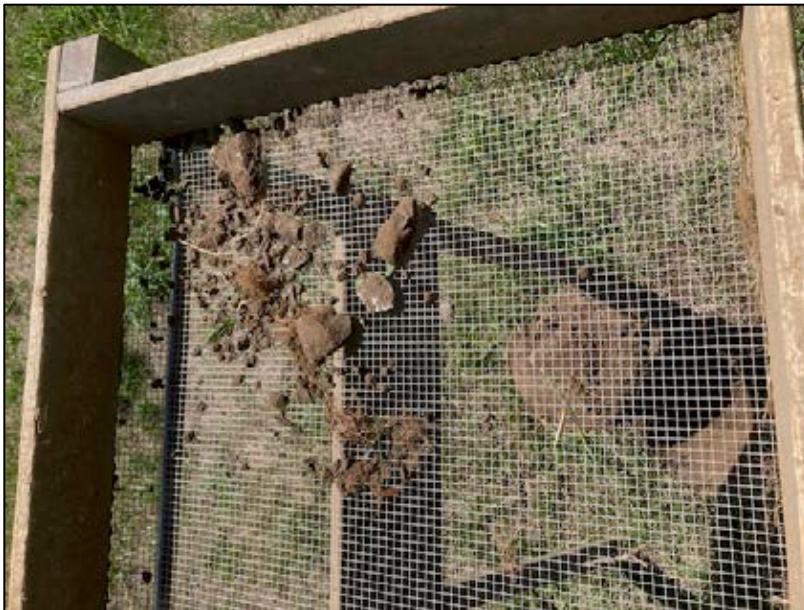
Image 6: Representative image of gravel/construction debris fills found in test pits.
