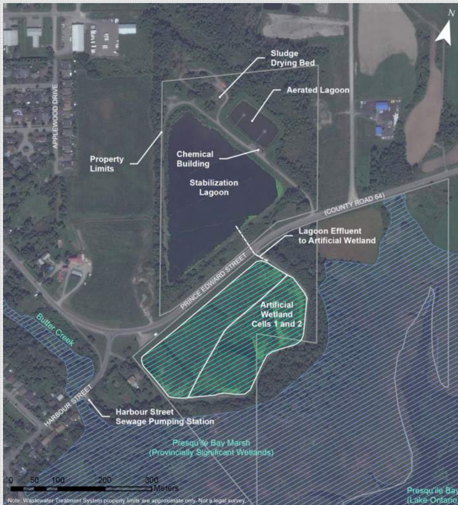
Figure 2 – Brighton Lagoon Treatment System Site Plan
