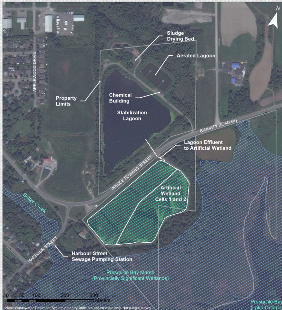
Figure 2 – Brighton Lagoon Treatment System Site Plan
